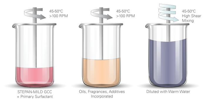
A unique mixing procedure is employed to form this multilamellar vesicle system. STEPAN-MILD GCC and other surfactants are premixed together. Oils, fragrances, and other additives are then introduced followed by dilution with warm water and high shear mixing. Lastly, the material being suspended is added and mixed gently to avoid aeration.
